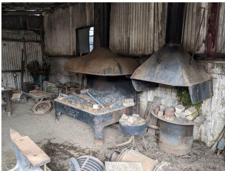
Interior of the Blacksmith's Shop illustrating Allday and smaller forges.
